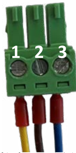
[Fig. 7] RS232 terminal with wires inserted
