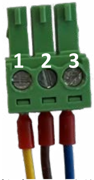
[Fig. 7] RS232 terminal with wires inserted
