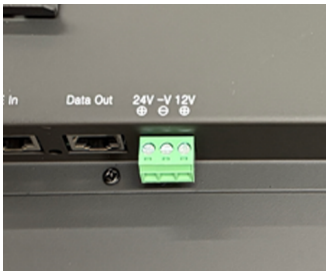
[Fig. 9] 12/24VDC terminal
