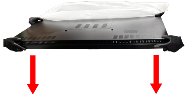
[Fig. 1] Lay display down evenly on both sides
