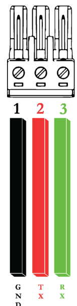
[Fig. 7] RS232 terminal with wires inserted
