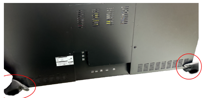
[Fig.4] Bottom display support and vertical transport
