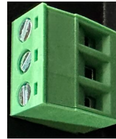
[Fig. 9] 12/24VDC terminal
