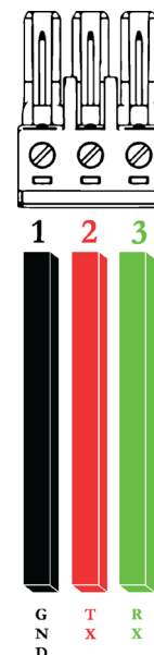
[Fig. 7] RS232 terminal with wires inserted
