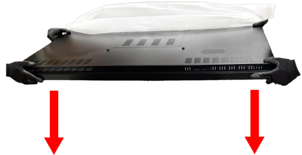
[Fig. 1] Lay display down evenly on both sides
