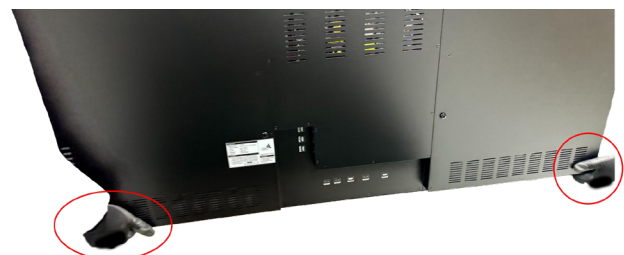
[Fig. 4] Bottom display support and vertical transport
