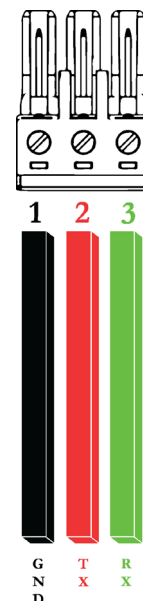
[Fig. 7] RS232 terminal with wires inserted
