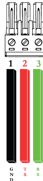
[Fig. 7] RS232 terminal with wires inserted
